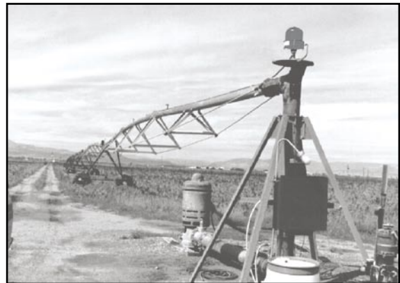
NI Electric Pivot Conversion, including pivot panel with options, collector ring, & accessories.
