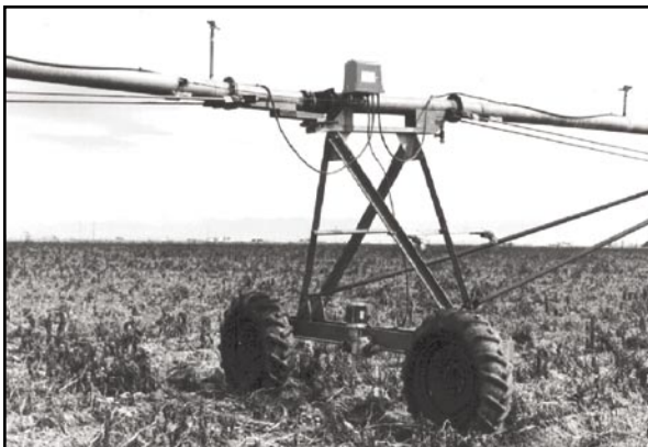
NI Electric Drive & Control Conversion utilizing existing system base deck and structure.
